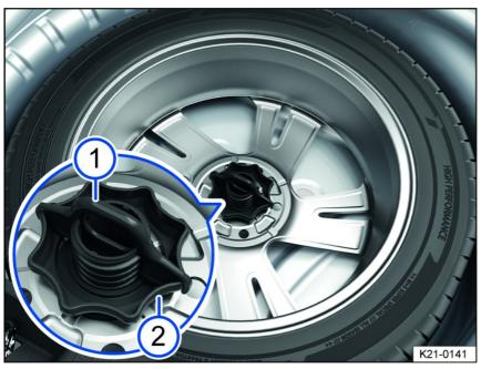
Fig. 205 In the luggage compartment: handle to secure the compact spare wheel.
