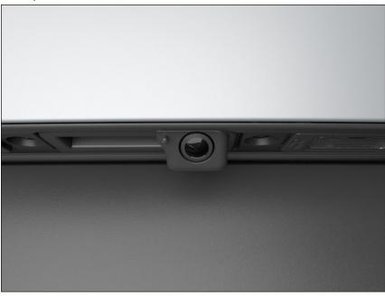
Fig. 213 In the rear of the vehicle: Rear View Camera system on the handle (general example).
