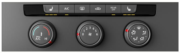
Fig. 106 In the upper section of the center console: Climate control bar for the manual climate control system.
