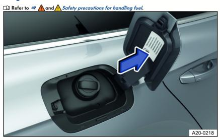
Fig. 168 On the inside of the fuel filler flap: fuel label (general example)
