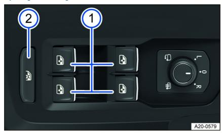
Fig. 70 In the driver door: Power window buttons.
