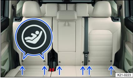
Fig. 39 On the second-row seats: Designation and symbol showing the ISOFIX/lower LATCH anchorage points for child restraints.
