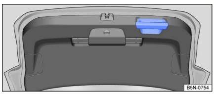
Fig. 64 In the open trunk lid: handle for closing the trunk lid.
