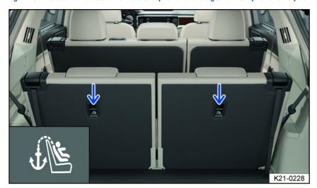
Fig. 42 On the back of the third-row seats: Top tether anchorages for the top tether safety belt.
