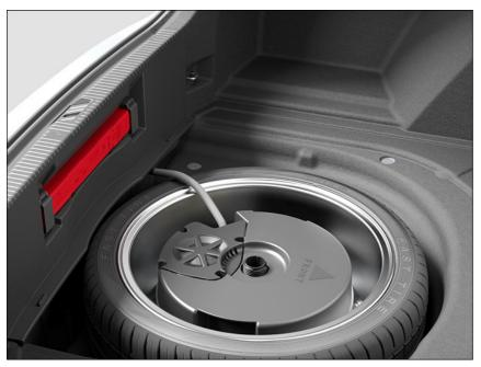
Fig. 203 Removing the subwoofer.
