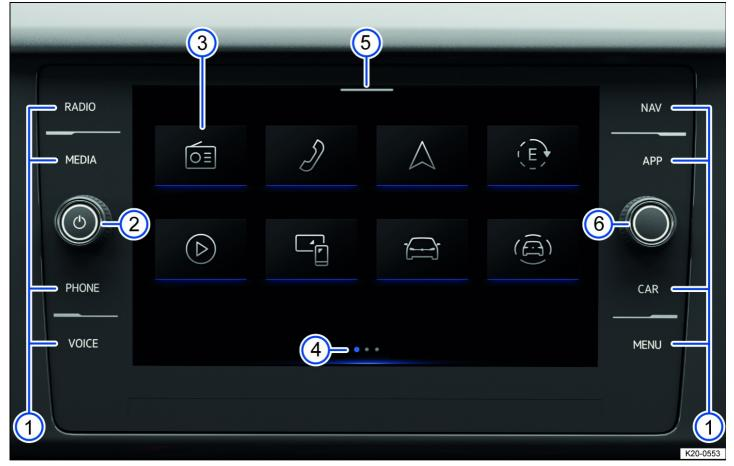
Fig. 156 Overview: display and control unit, 8" version.
