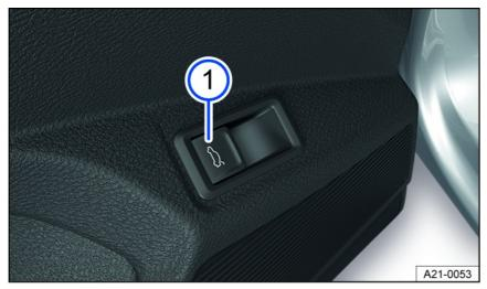
Fig. 65 In the driver door: Button for power opening the trunk lid.
