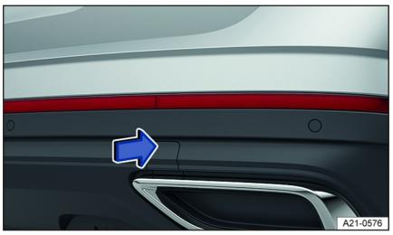
Fig. 184 In the right rear bumper: Remove cover.
