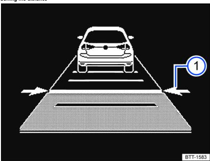
Fig. 133 In the instrument cluster display: set distance (1) (general example, ACC is regulating).
