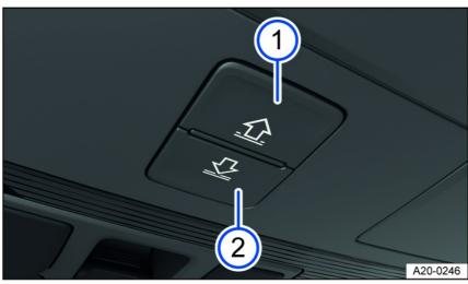
Fig. 103 In the headliner: buttons for controlling the sunshade.
