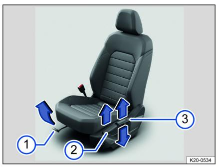
Fig. 74 On the driver seat: Controls.
