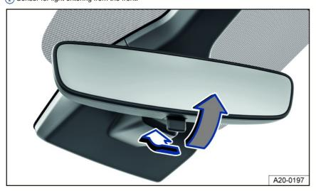
Fig. 100 On the windshield: manual dimming interior rearview mirror.
