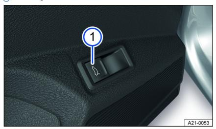
Fig. 59 In the driver's door: Button for powered opening of the trunk lid (general example).
