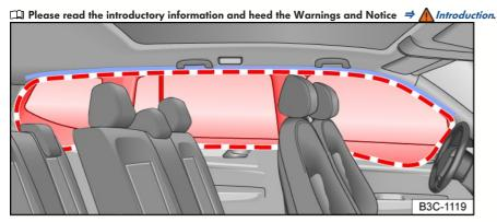
Fig. 37 On the left side of the vehicle: installation location and deployment zone of the Side Curtain Protection®.
