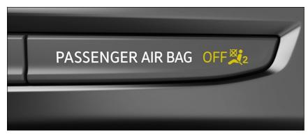
Fig. 32 In the center console: Indicator light for the deactivated front passenger's front airbag.
