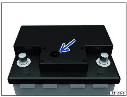
Fig. 196 On the top of the 12 V vehicle battery: Window (general example).
