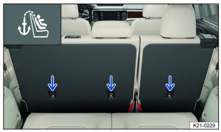
Fig. 41 On the back of the second-row seats: Top tether anchorages for the top tether safety belt.
