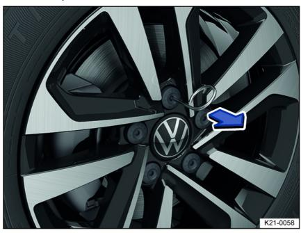
Fig. 201 Remove the caps from the wheel bolts.
