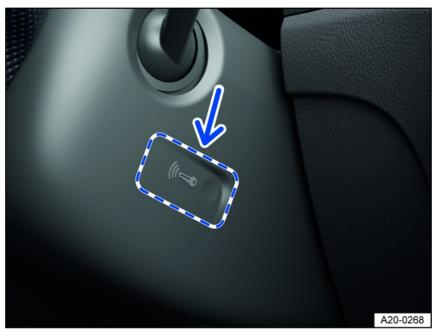
Fig. 113 On the right side of the steering column: emergency start function on vehicles with Keyless Access with push-button start.
