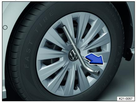
Fig. 200 Remove the wheel hub cover.
