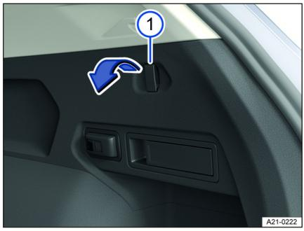
Fig. 166 In the luggage compartment: fold-out shopping bag hooks.
