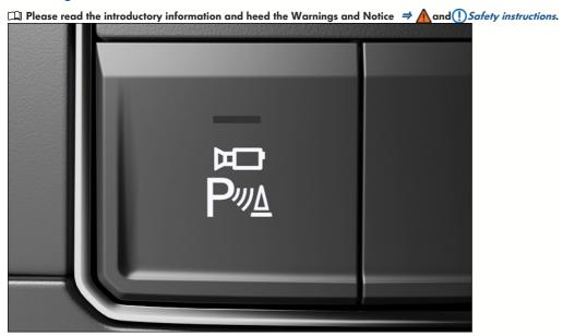
Fig. 145 In the center console: Button for switching the Area View on and off.
