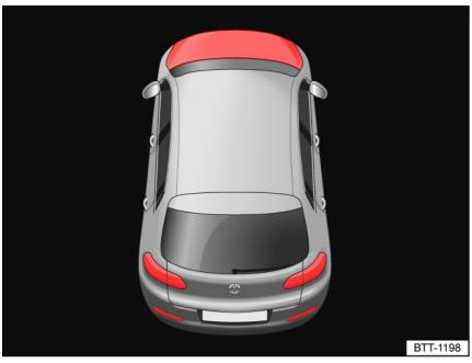
Fig. 188 In the instrument cluster display: the hood is open or not closed correctly (general example).
