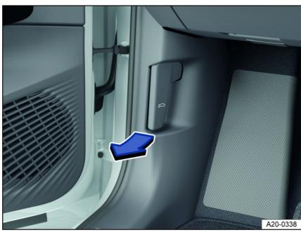
Fig. 186 In the driver's side footwell: Release lever for the hood (general example).
