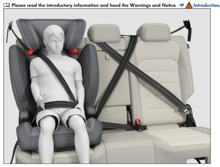
Fig. 47 Correctly fastened child on a booster seat.
