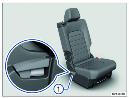
Fig. 80 Second row seats: folding the outer rear seats forward into the cargo floor position.
