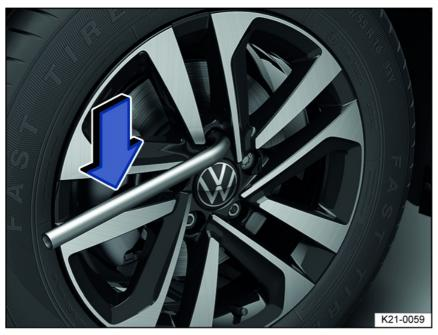
Fig. 202 Changing a tire: loosening the wheel bolts.
