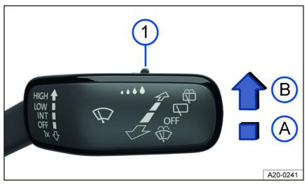
Fig. 98 On the right side of the steering column: windshield wiper lever.
