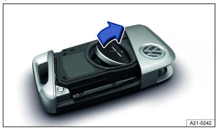
Fig. 55 Vehicle key: replacing the button cell battery
