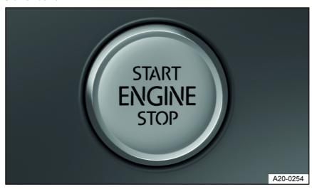
Fig. 111 In the lower area of the center console: starter button for starting the engine.
