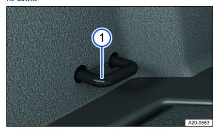
Fig. 163 In the luggage compartment: Tie-down (general example).
