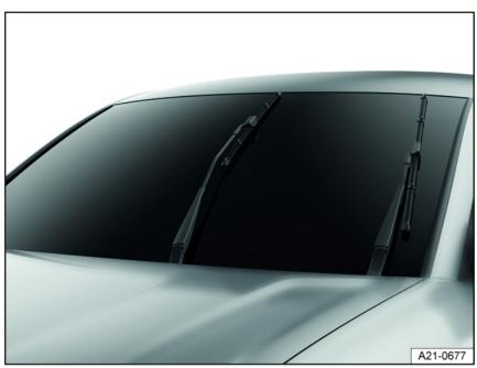
Fig. 171 Windshield wipers in service position (general example).
