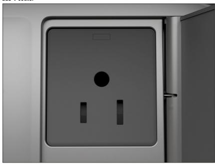
Fig. 154 In the center console at the rear: 115 V socket (depending on the vehicle equipment).
