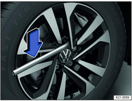
Fig. 209 Wheel change: removing wheel bolts with the lug wrench.
