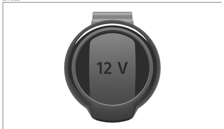
Fig. 153 In the lower part of the center console, at the rear of the center console or on the left-hand side of the luggage compartment: Hinged 12-volt socket (general example).
