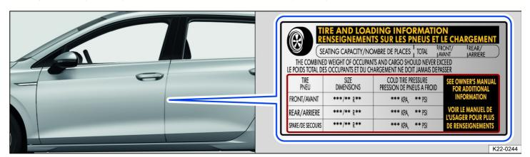
Fig. 197 On the driver door pillar: Tire inflation pressure label.
