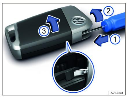
Fig. 54 Vehicle key: opening the battery compartment cover.
