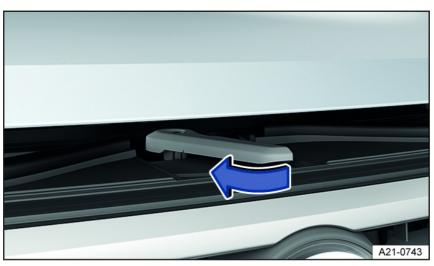
Fig. 187 Above the radiator grille: Opening lever for the hood.
