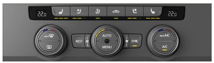
Fig. 105 In the upper section of the center console: Climate control bar for the Climatronic system.
