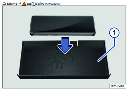
Fig. 158 Diagram: storage compartment with a liner pad for wireless charging.
