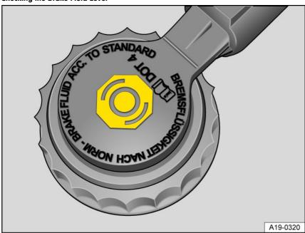
Fig. 194 In the engine compartment: cap on the brake fluid reservoir (version 1).
