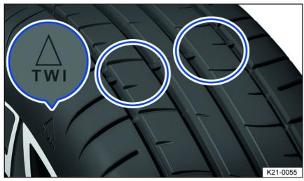
Fig. 199 Tire tread: tread wear indicator.
