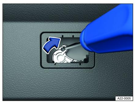
Fig. 69 In the luggage compartment: trunk lid emergency release.
