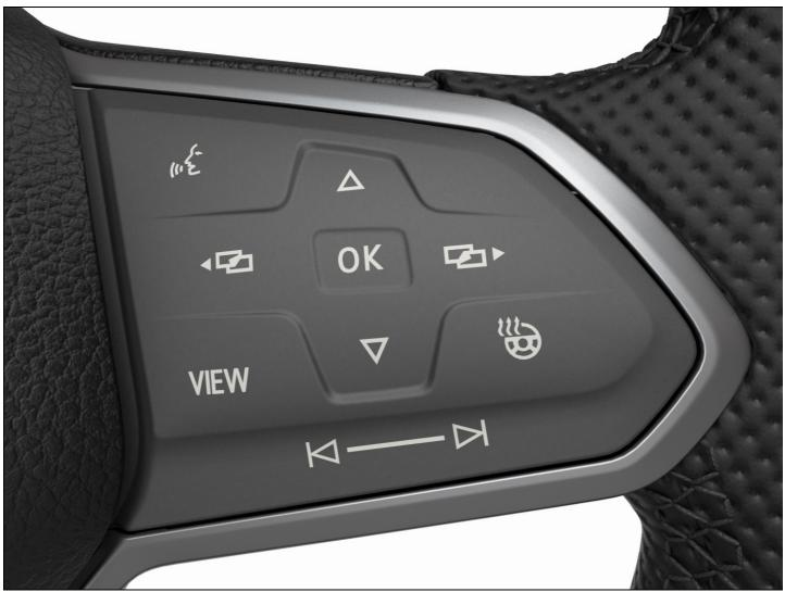
Fig. 17 Right side of the multi-function steering wheel: Operating the analog instrument cluster (variant 2).
